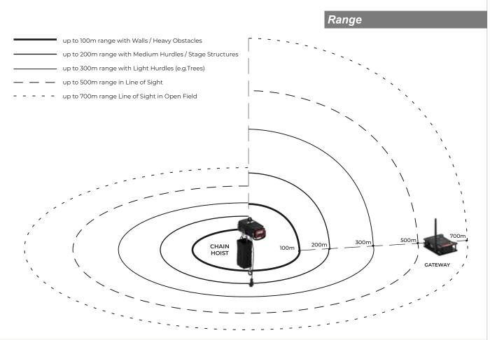
The maximum range of any wireless system depends on the propagation conditions. If the propagation between the Chain Hoists and the Gateway is in line of sight, the maximum range achievable with our system is about 600 meters. In the graph we have simulated the limitations due to various types of obstacles. Data are taken from field tests and theoretical calculations and are intended for guidance. Actual performance will be determined by site conditions.
