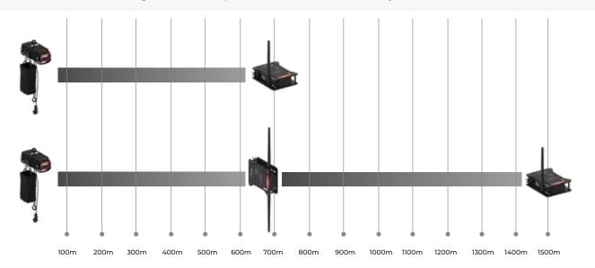
In case it is necessary to cover longer distances or there are large obstacles to overcome, it is possible to add Repeaters, which can be located as far as 600 meters from the cells and 700 meters from the Gateway. It is not possible to connect multiple Repeaters in series: each Repeater needs a direct connection to the Gateway.
